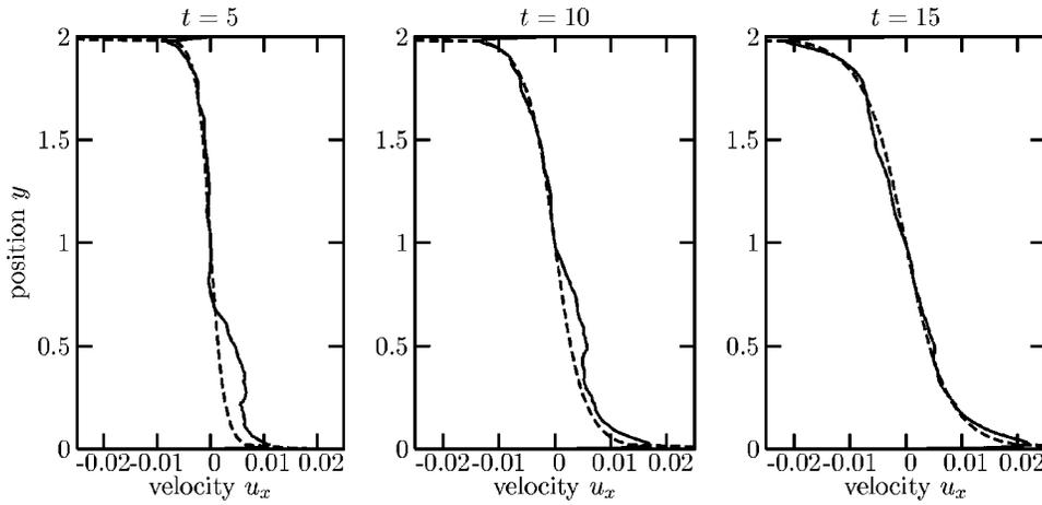
FIG. 3. Velocity profile at  $x=0$  and different instants of time. —, Numerical results; ---, analytical asymptotic approximation (nondimensional values).
