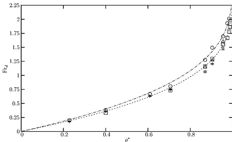
FIG. 7. Froude number of the dense front  $Fr_d$  vs  $\varrho^*$  in experiments and numerical simulations for both viscosity models. For symbols see Fig. 6; ---,  $2\sqrt{2}[1-(1-\varrho^*)^{0.3}]$ ; -.-,  $1.8\sqrt{2}[1-(1-\varrho^*)^{0.3}]$ .
