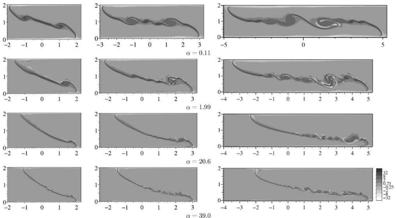
FIG. 10. Nondimensional vorticity maps for different density ratios and at different stages in the flow development for the constant dynamic viscosity model  $\lambda(\Phi)=1$ . The dense front positions are taken the same for the three density ratios.
