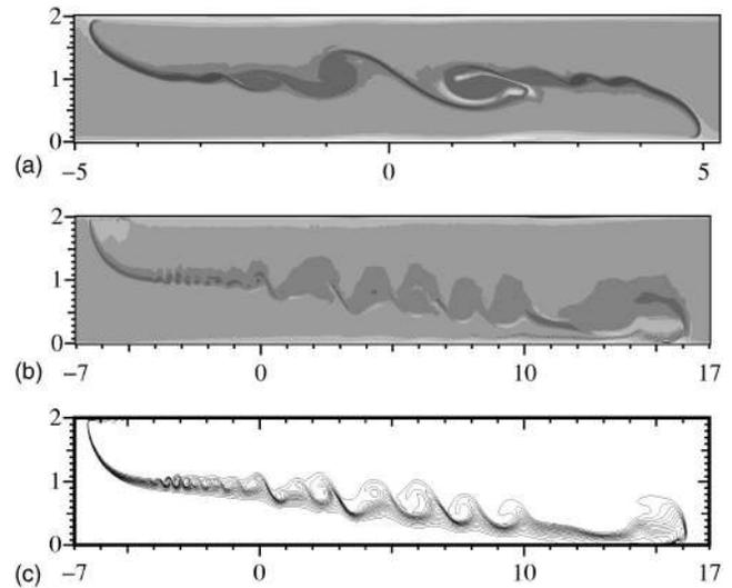
FIG. 11. (a,b) Nondimensional vorticity maps for the steady flow (long times). (a)  $\alpha=0.11$ ,  $Re=4.80 \times 10^3$  at nondimensional time  $t=8$  ( $\bar{t}=3$  s); (b)  $\alpha=20.6$ ,  $Re=5.47 \times 10^4$  at nondimensional time  $t=46$  ( $\bar{t}=1.3$  s). See Fig. 10 for the gray scale legend. (c) Nondimensional density isolines,  $\alpha=20.6$ ,  $Re=5.47 \times 10^4$  at nondimensional time  $t=46$  ( $\bar{t}=1.3$  s).
