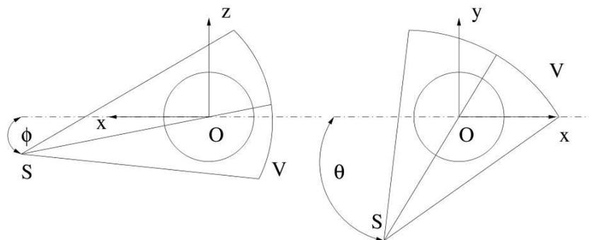
**Figure 1.** Scheme of the data acquisition geometry.  $(\mathbf{O}; x, y, z)$  defines the Carrington heliocentric frame of reference.  $S$  is the spacecraft considered.  $\phi$  is the latitude, and  $\theta$  the longitude of this spacecraft.  $V$  is the virtual detector.
