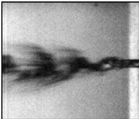
FIGURE 10. Instantaneous initial breakup image,  $D_l = 0.32$  mm,  $U_g = 165$  m s<sup>-1</sup>,  $U_l = 16.5$  m s<sup>-1</sup>,  $We = 116$ ,  $Re_g = 1.1 \times 10^5$ ,  $Re_l = 5280$ ,  $m = 0.07$ ,  $M = 0.12$ .
