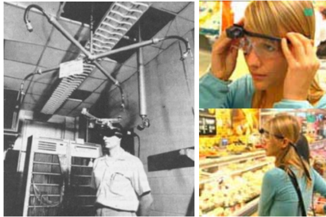
Figure 2.4: Left : Early head-mounted display device developed by Ivan Sutherland at Harvard University, 1967. Right : Example of a wearable head-mounted eye tracking system (from www.eye-square.com )
