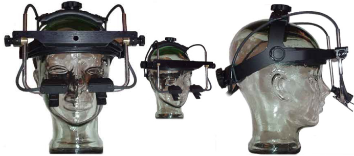
Figure 2.1: Typical eye tracking system using head mount. Model presented SR Research EyeLink II
