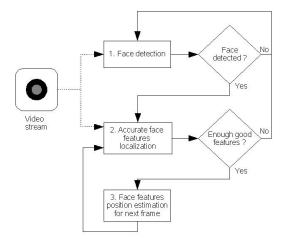
Figure 2. General architecture of the face and eye/gaze tracking algorithm.
