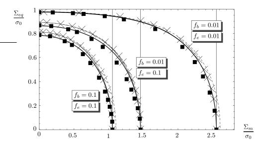
Figure 3. Effective yield surface for a porous material with two populations of voids for different void volume fractions  $f_b$  (small voids) and  $f_e$  (large voids). Upper bound (8) (crosses), estimate (14) with (13) and (12) (black solid line), estimate (14) with (13) and (17) (thick black solid line), FEM simulations (full squares), hydrostatic point of [14] (vertical line), Gurson yield function with total porosity f (dashed line).
