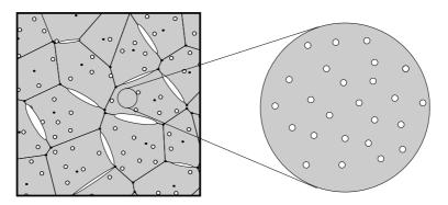
Figure 1. Left: polycrystalline structure of  $UO_2$  showing intergranular lenticular and intragranular voids. Right: close-up on the spherical intragranular voids.
