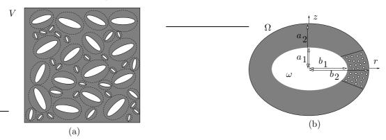
Figure 2. (a) Assemblage of ellipsoids. (b) Single hollow ellipsoid.
