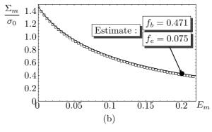
Figure 5. Macroscopic response of a porous hollow sphere under hydrostatic loading. Full circles: upper bound (10); Black Solid Line: estimate (14). White Squares: modified secant method (100 layers surrounding the cavity  $\omega$ ; a local porosity  $f_b^i$  is defined in each layer). (a) Initial porosities:  $f_b = 0.1$ ,  $f_e = 0.2$ . (b) Initial porosities:  $f_b = 0.1$ ,  $f_e = 0.01$ .
