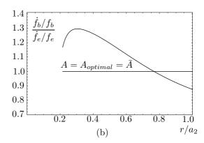
Figure 4. Hollow sphere under hydrostatic tension: relative rate-growth of the damage parameters. Exact result (Perrin [14], solid line; or equivalently N-phase secant method with  $N \geq 100$ ), predictions based on the  $A_{optimal}$  minimizing (8) (horizontal solid line) or on the approximation (9) (horizontal dashed line). (a)  $f_e = 1$  %,  $f_b = 10$  %. (b)  $f_e = 1$  %,  $f_b = 1$  %.
