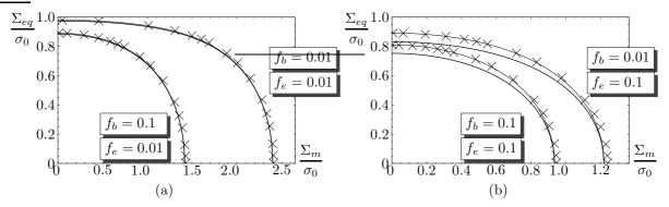
Figure 6. Effective yield surface of a Gurson material  $(q_1=q_3=1)$  containing randomly oriented oblate ellipsoidal voids (w=1/5). Comparison between the upper bound (28) (crosses), the estimate (14) (solid line) with (31) and (33) and the estimate (14) (thick solid line) with (33) and (15) where  $\widetilde{\mu}_1$  is estimated with the PCW bound [16].
