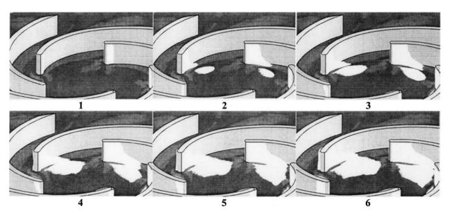
Fig. 13 Development of the two-phase areas as NPSH decreases (corresponding to points on Fig. 12)
