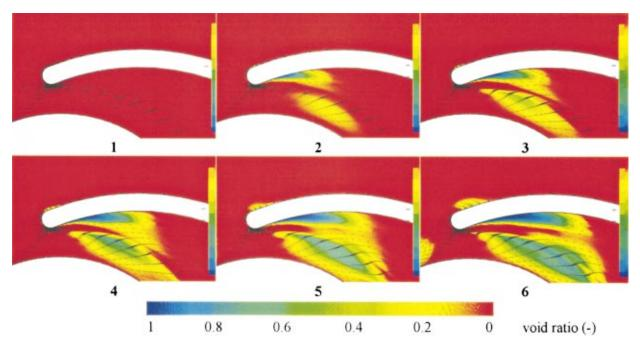
Fig. 14 Void ratio evolution on a blade-to-blade surface close to the shroud, and velocity fields (corresponding to the NPSH decrease represented on Fig. 12)
