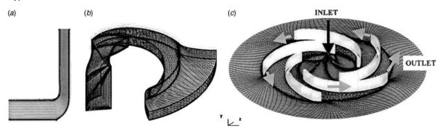
Fig. 9 Mesh applied for the calculations (300,000 cells). (a) Meridional view, (b) three-dimensional view of a blade-to-blade channel, (c) view of the mesh on hub side of the pump. (The entire pump geometry is reconstructed by rotation of the single blade-to-blade channel.)
