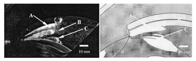
Fig. 15 Vapor structures on suction side (experiment NPSH=8 m, computation NPSH=7 m). Calculation: iso-density contour ( $\rho \approx 0.95 \rho_1$ : void ratio >5 percent) drawn in yellow, shroud in blue, blade in gray.
