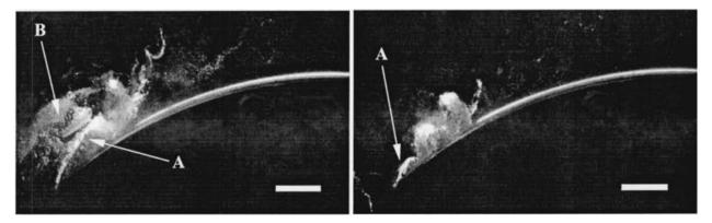
Fig. 4 Unsteady-state of blade cavitation on pressure side at two different time and NPSH=7 m (laser light sheet)
