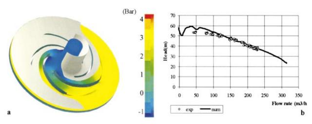
Fig. 11 (a) Total pressure elevation in the pump (nominal flow rate), (b) characteristics H(Q) of the pump in noncavitating conditions
