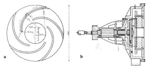
Fig. 1 (a) Impeller geometry, (b) housing
