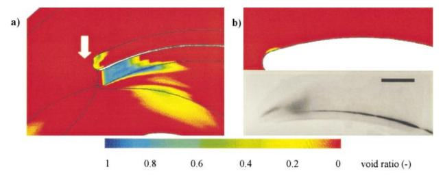
Fig. 16 (a) Numerical void ratio distribution, (b) pressure side cavity, comparison with experiment (NPSH=7 m)
