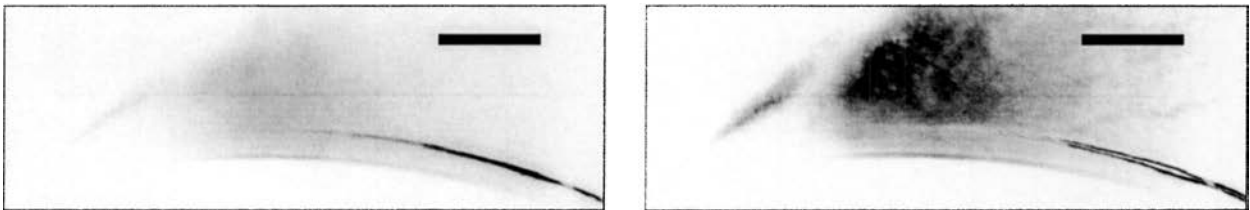
Fig. 6 Mean vapor distribution and standard deviation on pressure side, Qn, NPSH=6 m
