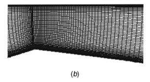
Fig. 2 (a) Curvilinear-orthogonal mesh of the Venturi-type section (160 $\times$ 50 cells).  $L_{\rm ref}=$ 224 mm. (b) Zoom in the throat region.
