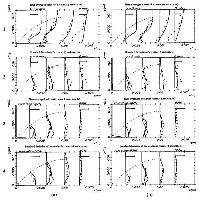
Fig. 7 Time-averaged values and standard deviation of velocity (1,2) and void ratio (3,4). Numerical results: (a) modified k- $\varepsilon$ , (b) compressible k- $\omega$  (lines) and optical probe measurements (points)— $V_{\rm ref}$ =7.2 m/s. Mean cavity length 45 mm: dotted line =experimental external shape of the cavity, obtained from image processing (sigma=2.4).
