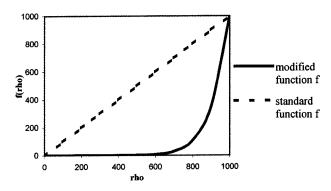
Fig. 4 Modification of the mixture viscosity (n=10)
