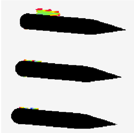
Figure 19. Numerical simulation of the unsteady cavitating behaviour of the cascade of hydrofoils (see animation ).
