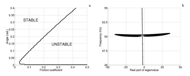
Figure 8 : Stability and complex eigenvalues as a function of angle  $\theta$  and brake friction coefficient. Coupled resonant frequencies between 50-51 Hz.
