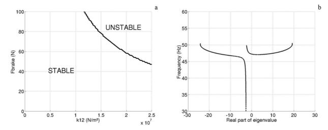
Figure 12 : Stability and complex eigenvalues as a function of stiffness  $k_{12}$  and force  $F_{brake}$ . Coupled resonant frequencies between 47-47 Hz.
