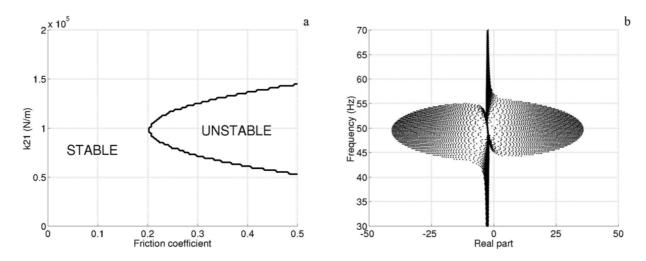
Figure 9 : Stability and complex eigenvalues as a function of stiffness  $k_{21}$  and brake friction coefficient. Coupled resonant frequencies between 45-58 Hz.
