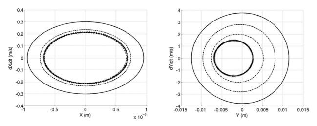
Figure 17 : X-limit cycle and Y-limit cycle for  $\overline{\mu} = \mu_0 / 1000$  as a function of brake force  $F_{brake}$  (-----  $F_{brake} = 10N$ , -----  $F_{brake} = 10N$ , -----
