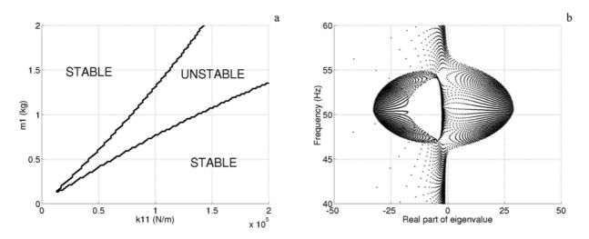
Figure 5 : Stability and complex eigenvalues as a function of mass  $m_1$  and stiffness  $k_{11}$ . Coupled resonant frequencies between 47-57 Hz.
