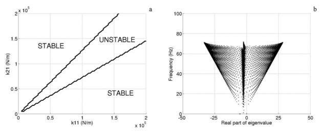
Figure 7: Stability and complex eigenvalues as a function of stiffness  $k_{21}$  and stiffness  $k_{11}$ . Coupled resonant frequencies between 10-70 Hz.
