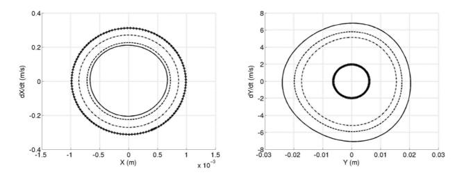
Figure 15 : X-limit cycle and Y-limit cycle for  $\overline{\mu} = \mu_0 / 1000$  as a function of angle  $\theta$ ( +++++  $\theta = 0.1$ rad., ----- $\theta = 0.3$ rad., -----  $\theta = 0.4$ rad., -----  $\theta = 0.5$ rad)
