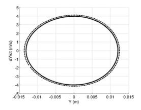
Figure 14 : Y-limit cycle for  $\overline{\mu} = \mu_0 / 1000$  ( — Original system, … Center manifold approach)
