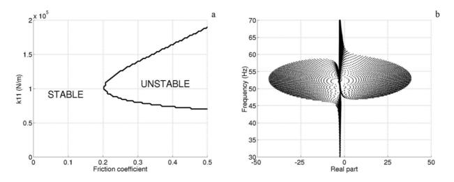
Figure 11 : Stability and complex eigenvalues as a function of stiffness  $k_{11}$  and brake friction coefficient. Coupled resonant frequencies between 48-52 Hz.
