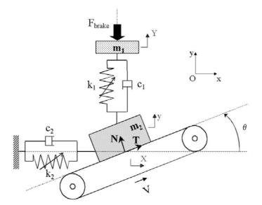
Figure 2 : Dynamic model of braking system
