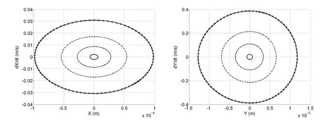
Figure 16 : X-limit cycle and Y-limit cycle for  $\overline{\mu} = \mu_0 / 1000$  as a function of non-linear stiffness coefficient  $k_{12}$  (+++++  $k_{12} = 10^7 N / m^2$ , -----  $k_{12} = 1.510^7 N / m^2$ , -----  $k_{12} = 2.510^7 N / m^2$ , -----  $k_{12} = 10^8 N / m^2$ )
