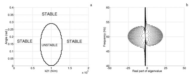
Figure 10 : Stability and complex eigenvalues as a function of angle  $\theta$  and stiffness  $k_{21}$ . Coupled resonant frequencies between 47-54 Hz.
