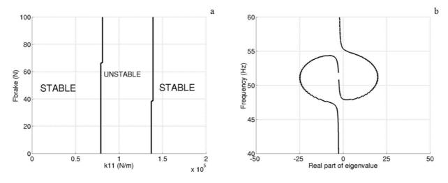
Figure 6 : Stability and complex eigenvalues as a function of force  $F_{brake}$  and stiffness  $k_{11}$ . Coupled resonant frequencies between 47-48 Hz and 55-56 Hz.
