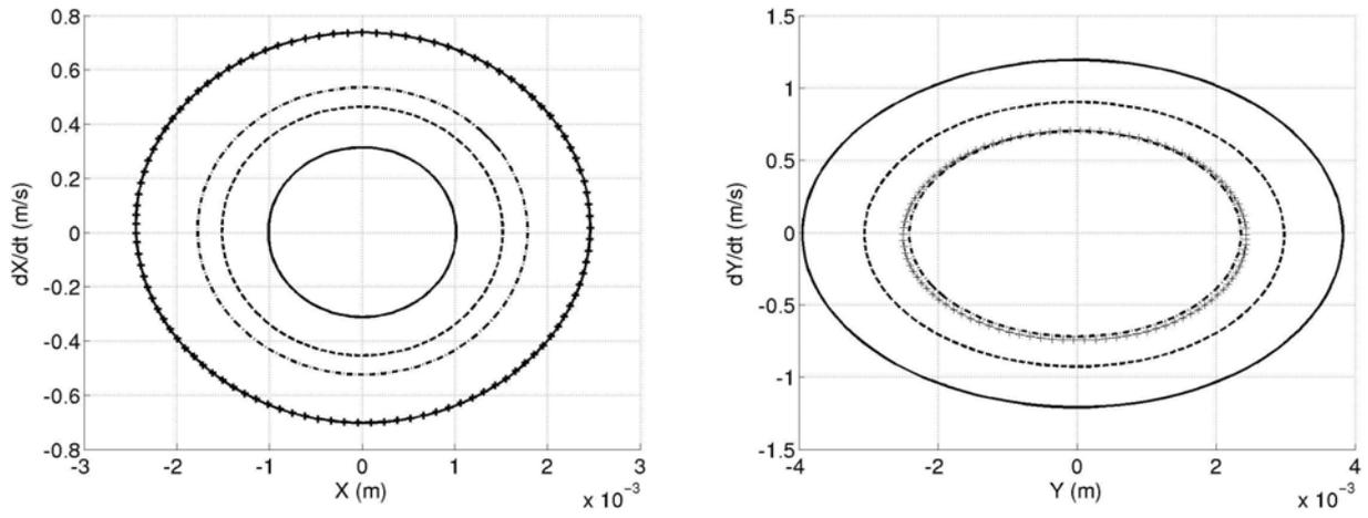
Figure 18 : X-limit cycle and Y-limit cycle for  $\bar{\mu} = \mu_0 / 1000$  as a function of mass  $m_1$
