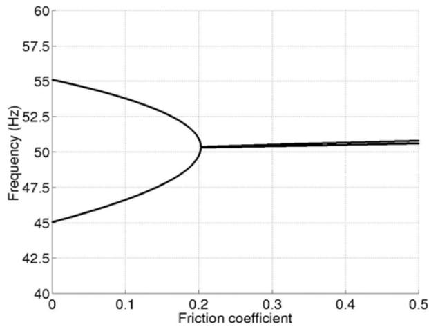
Figure 3 : Coupling of two eigenvalues
