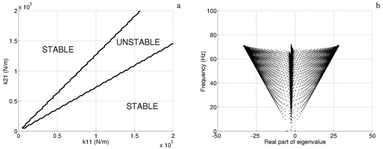
Figure 7: Stability and complex eigenvalues as a function of stiffness  $k_{21}$  and stiffness  $k_{11}$ .
