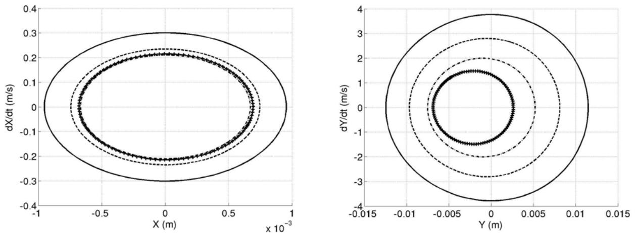
Figure 17 : X-limit cycle and Y-limit cycle for  $\bar{\mu} = \mu_0 / 1000$  as a function of brake force  $F_{brake}$  (—  $F_{brake} = 10N$ , ----  $F_{brake} = 10N$ , -----  $F_{brake} = 10N$ , +++++  $F_{brake} = 10N$ ).
