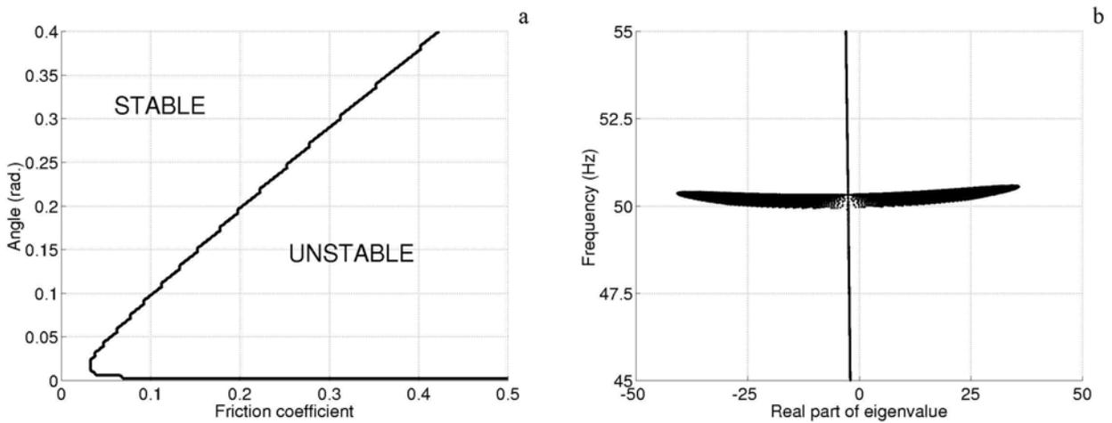
Figure 8 : Stability and complex eigenvalues as a function of angle  $\theta$  and brake friction coefficient.
