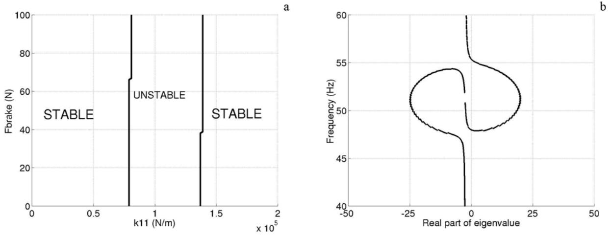
Figure 6 : Stability and complex eigenvalues as a function of force  $F_{brake}$  and stiffness  $k_{11}$ .
