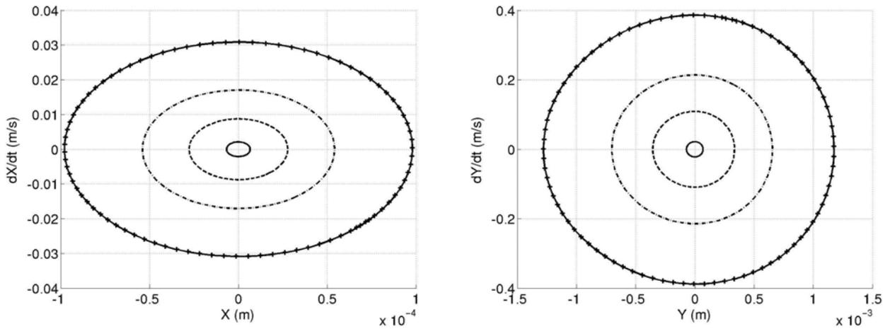
Figure 16 : X-limit cycle and Y-limit cycle for  $\bar{\mu} = \mu_0 / 1000$  as a function of non-linear stiffness coefficient  $k_{12}$  ( +++++  $k_{12} = 10^7 N/m^2$ , -----  $k_{12} = 1.510^7 N/m^2$ , ----  $k_{12} = 2.510^7 N/m^2$ , —  $k_{12} = 10^8 N/m^2$ )
