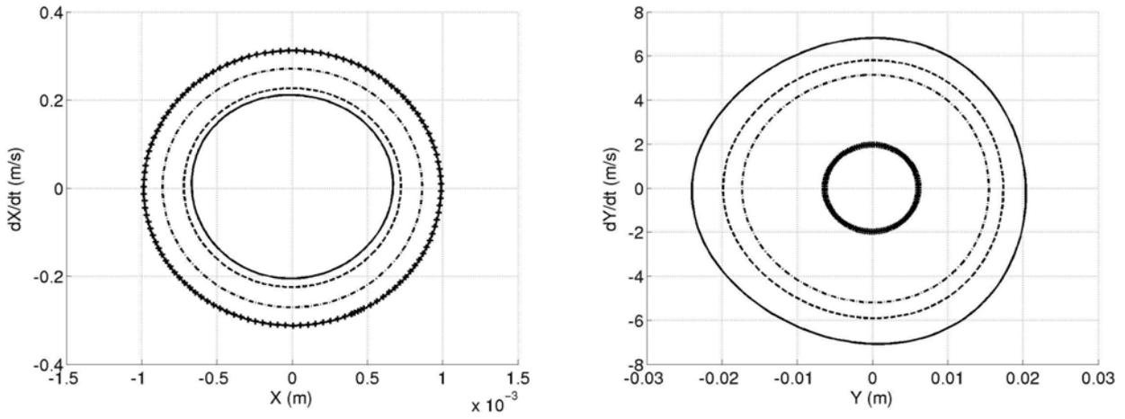
Figure 15 : X-limit cycle and Y-limit cycle for  $\bar{\mu} = \mu_0 / 1000$  as a function of angle  $\theta$
