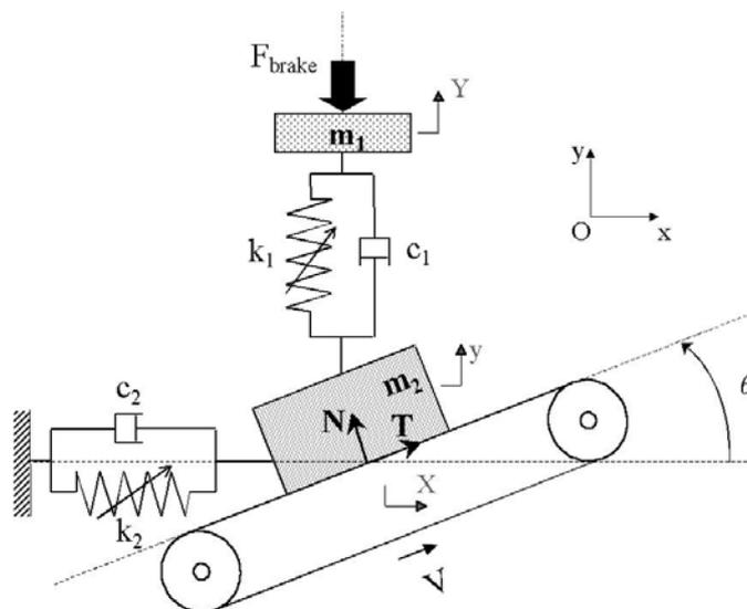
Figure 2 : Dynamic model of braking system
