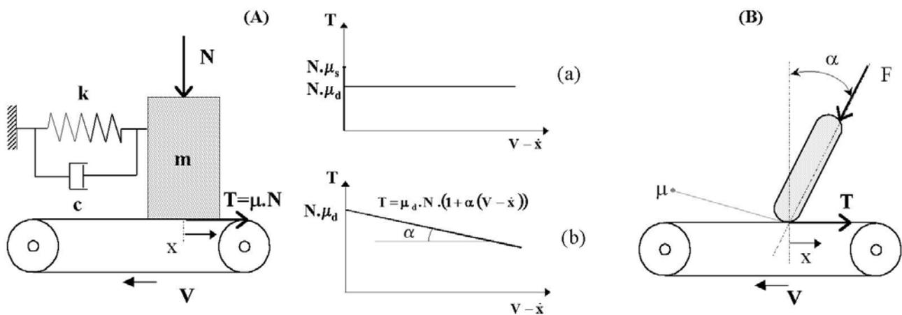
Figure 1 : Stick-slip and sprag-slip models
