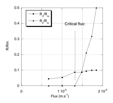
Fig. 8: Evolution of reversible,  $R_{\rm rf},$  and irreversible,  $R_{\rm if},$  fouling resistance vs. flux.
