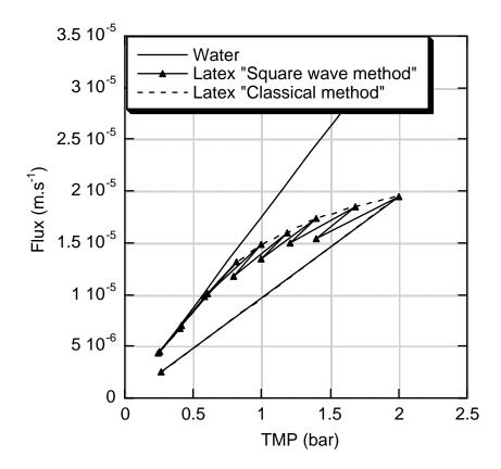
Fig. 5: Flux vs. TMP for the "square wave" technique; PVC latex,  $Qc = 0.79 \text{ m.s}^{-1}$ , [KCl] =  $10^{-3} \text{ M}$ .
