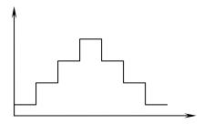
Fig. 1: Filtration procedure with flux stepping used in literature [1] to find the critical flux.
