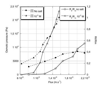
Fig. 11: Evolution of Rf/Rm and Rif/Rm and osmotic pressure for two different states of destabilization of particles; different ionic strength, crossflow velocity = 0.6 m.s<sup>-1</sup>, [latex] = 0.6 g.L<sup>-1</sup>.
