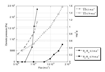
Fig. 10: Evolution of resistances and decomposition in term of osmotic pressure and irreversible resistance for two crossflow velocities; [latex] =  $0.6 \text{ g.L}^{-1}$  [KCI] =  $10^{-3} \text{ M}$ .
