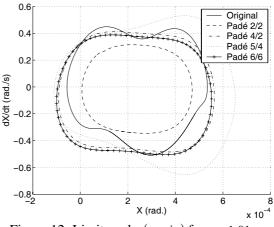
Figure 12: Limit cycle  $(\varphi_s, \dot{\varphi}_s)$  for  $\mu = 1.01\mu_0$
