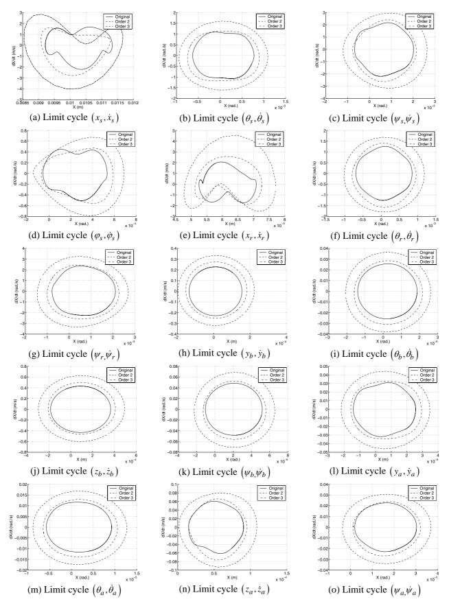
Figure 8: Comparison between the original system and the reduced system obtained by using the center manifold
