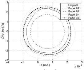
Figure 15: Limit cycle  $(\psi_r, \dot{\psi}_r)$  for  $\mu = 1.01\mu_0$
