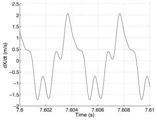
Figure 4 : Zoom of the axial velocity of the rotor  $(\mu = 1.01\mu_0)$
