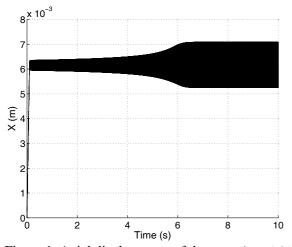
Figure 1: Axial displacement of the rotor ( $\mu = 1.01\mu_0$ )
