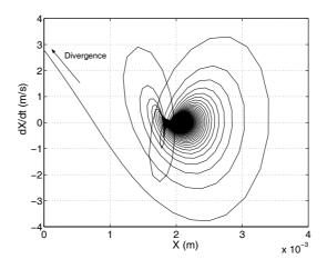
Figure 24: divergence for the limit cycle  $(x_s, \dot{x}_s)$
