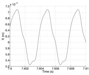
Figure 2: Zoom of the axial displacement of the rotor  $(\mu = 1.01\mu_0)$
