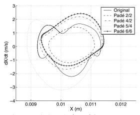
Figure 9: Limit cycle  $(x_s, \dot{x}_s)$  for  $\mu = 1.01\mu_0$
