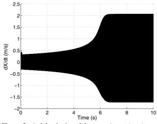
Figure 3 : Axial velocity of the rotor ( $\mu = 1.01\mu_0$ )
