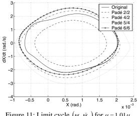
Figure 11: Limit cycle  $(\psi_s, \dot{\psi}_s)$  for  $\mu = 1.01\mu_0$
