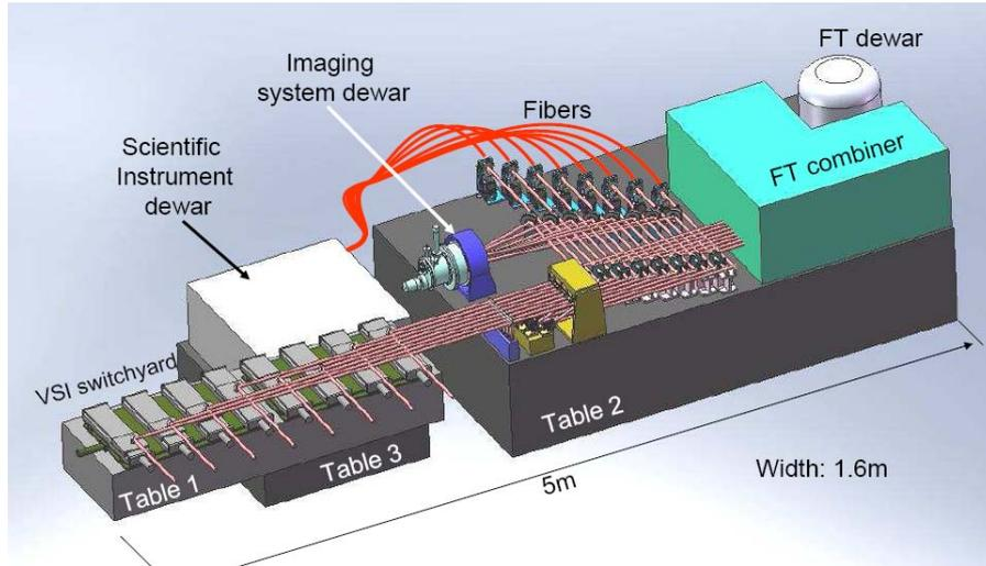
Fig. 3. General implementation of the VSI instrument
