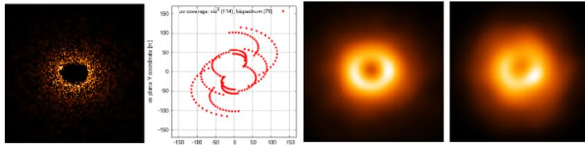
**Fig. 2.** VLTI/VSI image reconstruction simulation performed with 4 UTs on a model of a clumpy torus at the center of an AGN [5]. Left: model image; middle left: coverage of the spatial frequencies; middle right: model image convolved with a perfect beam corresponding to the maximum spatial resolution; right: image reconstructed from simulated VSI data using the Building Block method.
