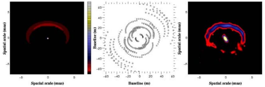
**Fig. 1.** Image reconstruction performed with 6 ATs on a model disk around an Herbig Ae star [4]. Left: model image; middle: coverage of the spatial frequencies; right: reconstructed image. The dust structure, the inner dust radius and the asymmetry (vertical structure) are well retrieved. Relative photometry is reliable (17% vs 19% of flux in the central star).
