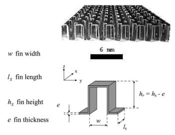
Fig. 3. Geometrical parameters of the OSF inserts.
