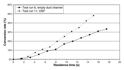
Fig. 9. Effect of geometrical configuration on reaction conversion rate.
