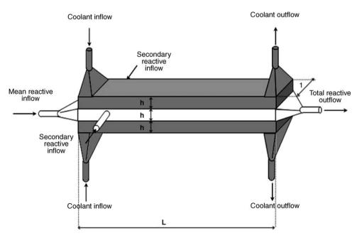
Fig. 1. Multifunctional heat exchanger.
