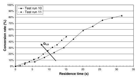
Fig. 8. Effect of reactive volume flow rate on. Reaction conversion rate with OSF.
