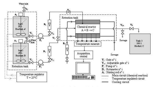
Fig. 2. Schematic diagram of the flow loop.
