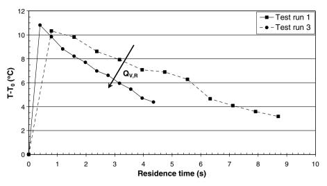
Fig. 5. Effect of coolant volume flow rate on reactive temperature rise in MHE.
