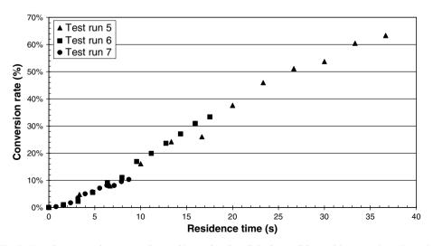
Fig. 7. Reactive conversion rate against residence time in adiabatic conditions with empty duct channel.
