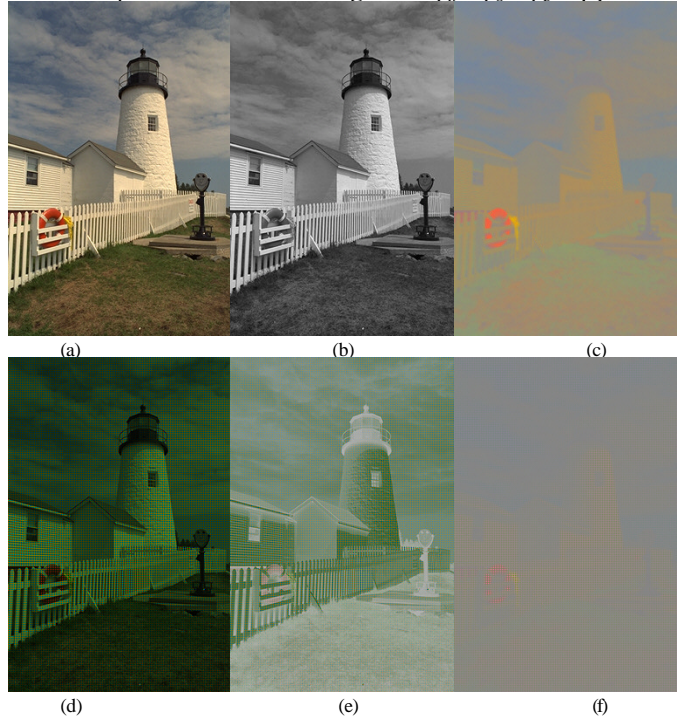
Figure 3: Decomposition of (a) a color image into (b) luminance and (c) chrominance as defined in eq. 5. (d) A CFA image with a single chromatic sensitivity per spatial location according to the Bayer CFA arrangement (the image appears greenish because of the double number of green pixels in the CFA). When subtracting luminance (b) from the CFA image (d), the resulting image is (e), which corresponds to a multiplexed version of sub-sampled chrominance. Selecting pixels in front of each color sample of the Bayer CFA (i.e. de-multiplexing opponent colors) results in image (f). Also, sub-sampling image (c) results exactly in image (f). Thus, image (c) can be recovered from (f) using interpolation.
