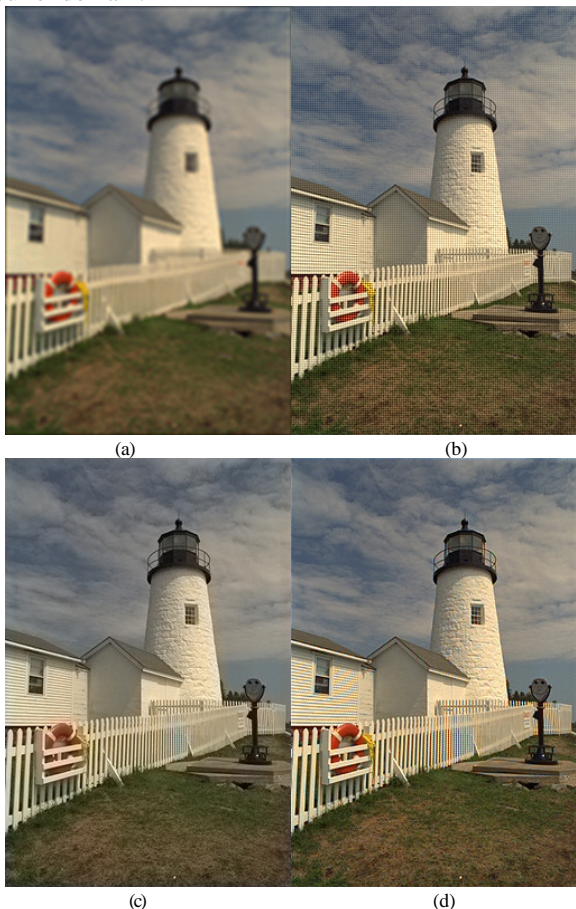
Figure 5: The four artifacts visible after demosaicing: (a) Excessive blurring (b) Grid effect (c) Watercolor (d) False color.
