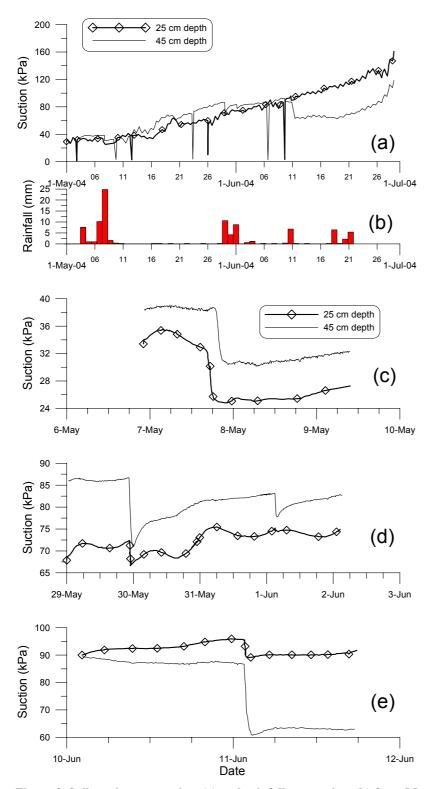
Figure 3. Soil suction versus time (a) and rainfall versus time (b) from May  $1^{st}$  2004 to July  $1^{st}$  2004. Details of soil suction versus time for rainfall periods (c, d, and e).
