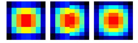
Figure 2: The approximate solution for conforming and non-conforming meshes. Left: conforming  $8 \times 6$  mesh, centre: non conforming  $4 \times 6, 4 \times 10$  mesh, right: conforming  $10 \times 10$ .
