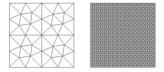
Figure 1: Regular conforming coarse and fine triangular grids
