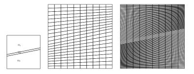
Figure 3: Domain and meshes used for the tilted barrier test: mesh 1 ( $10 \times 21$  centre), mesh 2 ( $10 \times 100$  right)
