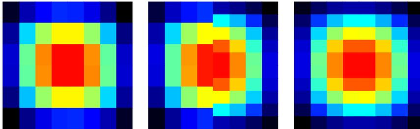
Figure 2: The approximate solution for conforming and non-conforming meshes. Left: conforming  $8 \times 6$  mesh, centre: non conforming  $4 \times 6, 4 \times 10$  mesh, right: conforming  $10 \times 10$ .
