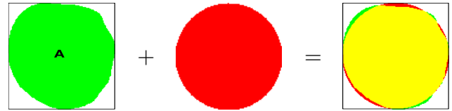
FIG. 5 – Principle of the correlation calculus : the cell to analyze (left) is correlated with the mean radius cell (middle) providing an geometric intersection (right).
