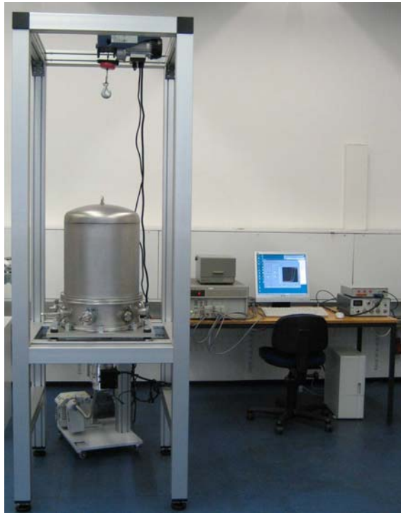
Figure 2. View of the vacuum system.
