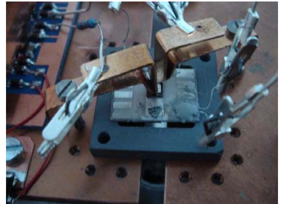
Figure 5. Detailed view of the sample ceramic substrate with electrical contacts. The heating coil is located below the substrate.
