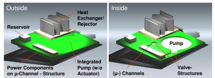
**Fig. 1 Outline of the integrated liquid cooling concept. All piping and pump emerge during board manufacture and SMT process.**
