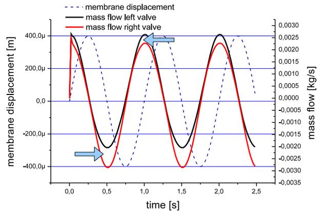
**Fig. 11 Simulation results: mass flow at inlet and outlet and sinusoidal membrane displacement with  $f=1$ Hz.**
