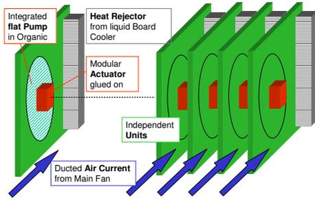
**Fig. 2 Possible arrangement of independent units for system cooling. As the units are flat, the air passes around them.**
