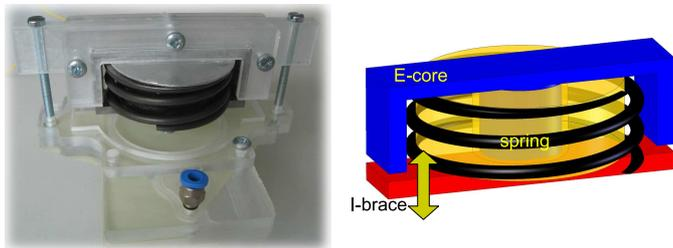
Fig. 6 Actuator with E-I core and spring to provide needed force in two directions.
