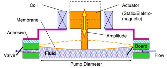
**Fig. 3 Schematic of pump with glued-on actuator. Further key features are valve and membrane characteristics.**
