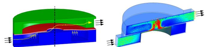
**Fig. 13 CAD model and CFD analysis of a membrane valve.**
