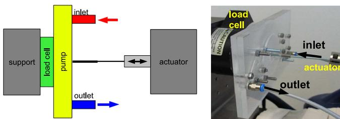
**Fig. 15** Test setup to measure flow rate of prototypes
