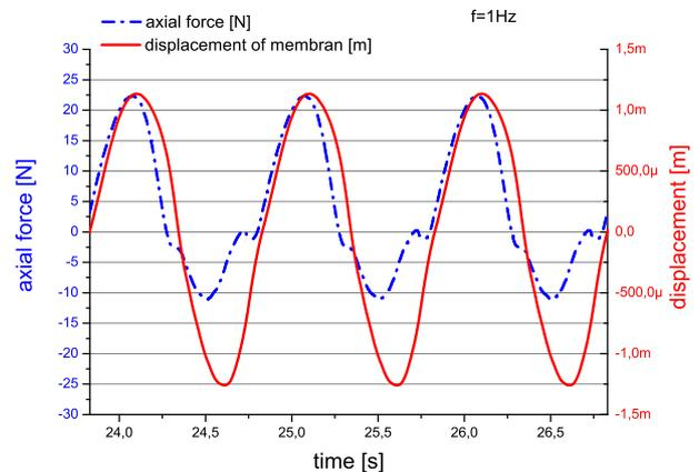
**Fig. 17** Measured axial force and displacement while excitation with  $f=1 \text{ Hz}$
