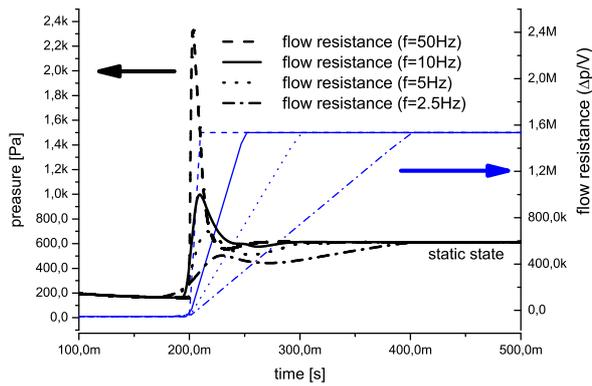
**Fig. 9 Dynamic behavior of tesla valves for different excitation frequencies (up to  $f = 50$  Hz).**
