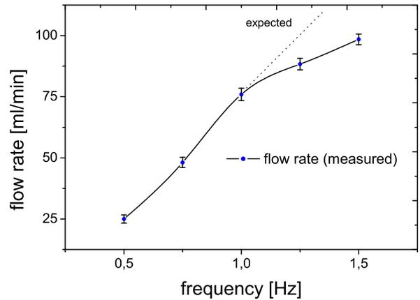
**Fig. 16** Measured flow rate as function of exciting frequency (membrane valves).
