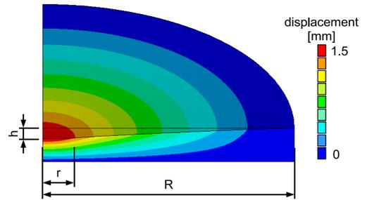
**Fig. 4 FE-model to estimate the displacement volume of an realistic membrane.**
