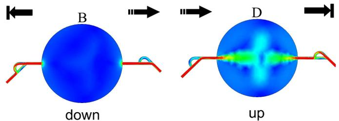
**Fig. 12 CFD analysis of membrane pump with tesla valves.**
