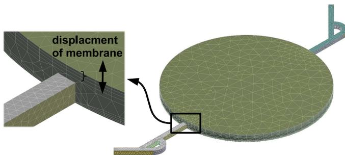
**Fig. 10 CFD analysis using moving mesh capability to simulate membrane displacement.**
