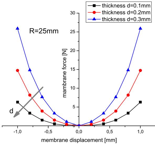
Fig. 5 Membrane force for different membrane thickness.
