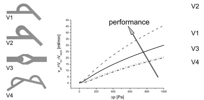
Fig. 8 Effective volume flow rate for different valve types (steady-state conditions).
