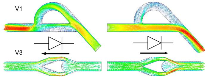
Fig. 7 Calculated velocity field in tesla valves. Flow resistance both for backward and forward flow can be derived.
