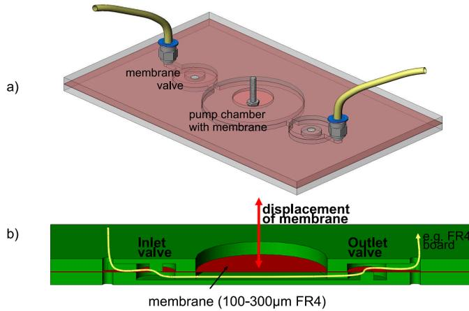
**Fig. 14** Prototype of pump a) with membrane valves, b) cross section of membrane pump.
