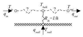
Figure 1. Inability of a resistive network to model a convective domain
