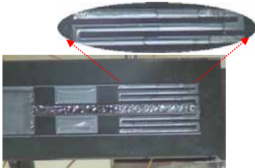
Fig.7 Flow pattern at the condenser near 5W of input power
