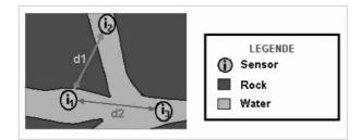
The distance d1 which separates the sensors i1 and i2 is shorter than the distance d2 which separates the sensors i1 and i3. However, the rock separating the couple of sensors (i1, i2) will degenerate the signal and will prevent sensor i2 from receiving the message correctly unlike i3.
