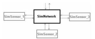
A SimSensor component simulates the sensor behavior. It possesses its own model and architecture. All the sensors have the same communication capabilities. They transmit their requests to the SimNetwork component sends this information to all sensors which can receive them, in the environment. Sim-Network can appear as the inference mecanism for the simulation.
