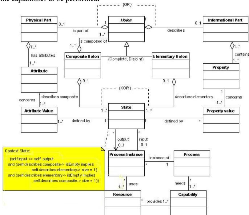
Fig. 3: Class diagram for the Holon model
