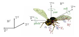
Fig. 1. Frames and wings angles
