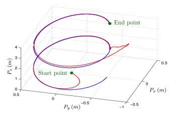
Fig. 4. The linear movement of the MAV in 3D (red), going from a start point to an end point, tracking a desired trajectory (blue), in presence of external disturbances applied at t = 20 s during 5 wingbeats.
