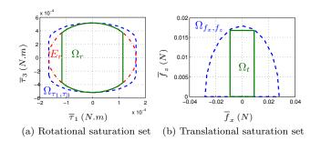
Fig. 3. Yaw torque versus roll torque (3a), defining the saturation set  $\Omega_{\tau_1,\tau_3}$  approximated to an ellipse  $E_r$  then to a set  $\Omega_r$ . Lift versus thrust (3b), defining the saturation set  $\Omega_{f_x,f_z}$  approximated to the set  $\Omega_t$ .
