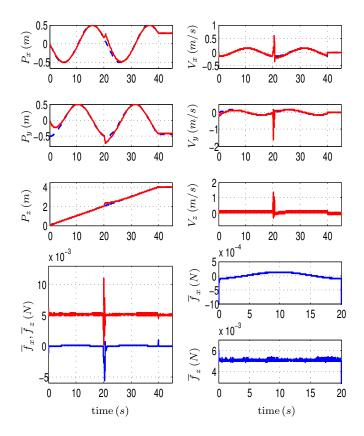
Fig. 5. The linear displacements, velocities (current in red and desired in blue) and corresponding control forces in presence of external disturbances applied at t = 20 s during 5 wingbeats. The control forces zoomed to 20 s to show the shape of the curves (bottom right).
