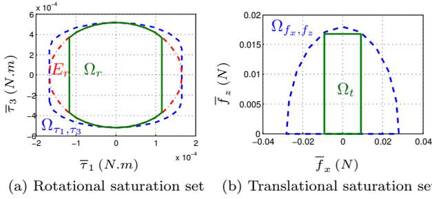
Fig. 3. Yaw torque versus roll torque (3a), defining the saturation set  $\Omega_{\tau_1, \tau_3}$  approximated to an ellipse  $E_r$  then to a set  $\Omega_r$ . Lift versus thrust (3b), defining the saturation set  $\Omega_{f_x, f_z}$  approximated to the set  $\Omega_t$ .
