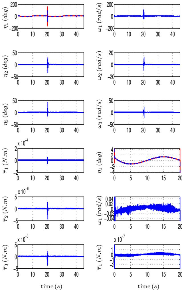
Fig. 6. The roll, pitch and yaw angles, angular velocities and control torques in presence of external disturbances applied at  $t = 20$  s during 5 wingbeats. The roll angle (current in red and desired in blue), angular velocity and control torque zoomed to 20 s to show the sinusoidal shape of the curves (bottom right).
