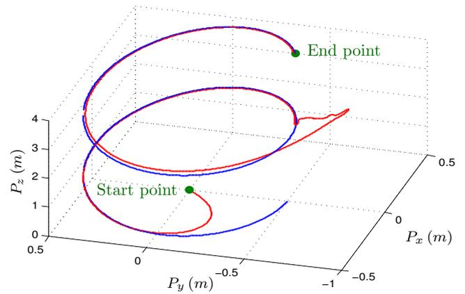
Fig. 4. The linear movement of the MAV in 3D (red), going from a start point to an end point, tracking a desired trajectory (blue), in presence of external disturbances applied at  $t = 20 \text{ s}$  during 5 wingbeats.
