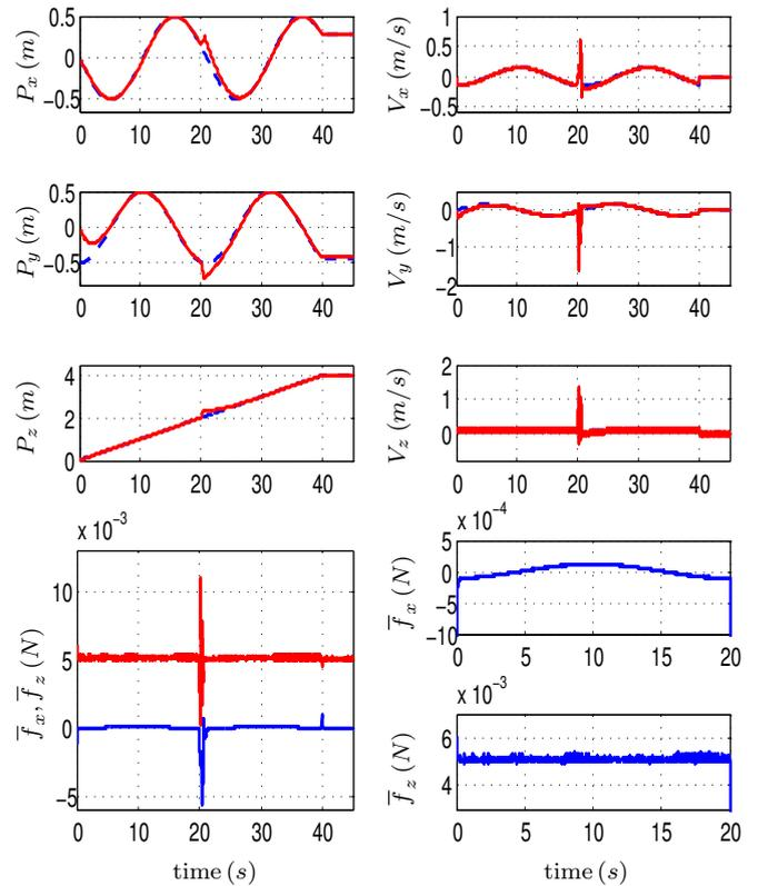
Fig. 5. The linear displacements, velocities (current in red and desired in blue) and corresponding control forces in presence of external disturbances applied at  $t = 20 \text{ s}$  during 5 wingbeats. The control forces zoomed to 20 s to show the shape of the curves (bottom right).
