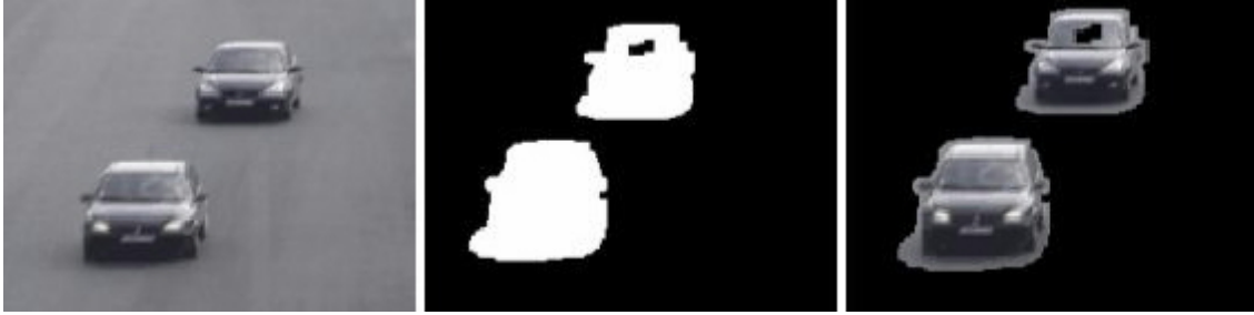
Figure 5. From left to right: current image, ROI mask, image to be compressed.
