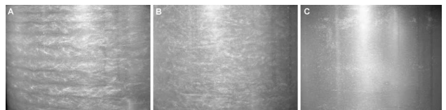
FIG. 1: Photographs of the flow at Re = 3.6 \times 10^3 . Left, A: only the inner cylinder rotating. Middle, B: counter rotating cylinders. Right, C: only the outer cylinder rotating. The flow structure is visualized using microscopic Mica-platelets (Pearlescence).
