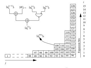
Fig. 1. The arrangement of 128 memory cells  $[q_k^{(j)}]_i$  and the hardware architecture of Eq. (4).
