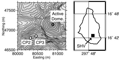
**Figure 1.** The position of the two tiltmeters located close to the dome at Soufrière Hills volcano (SHV), Montserrat [after Voight *et al.*, 1998]. CP3 is  $\sim 630$  m and CP2 is  $\sim 770$  m from the active vent. Contours increment at 50 m intervals, with both tiltmeters located at  $\sim 890$  m a.s.l. The area covered by the map is shown as a black square on the outline of Montserrat to the right.
