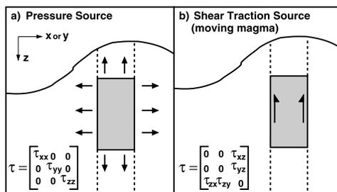
**Figure 2.** The two styles of deformation considered in this paper. (a) An isotropic pressurised conduit section representing an inflation of the conduit and (b) a shear traction model used to represent shear stresses at the wall of the conduit section, associated with vertical pressure gradients along the conduit. The stress tensor for each source is given at the bottom left of the panels.
