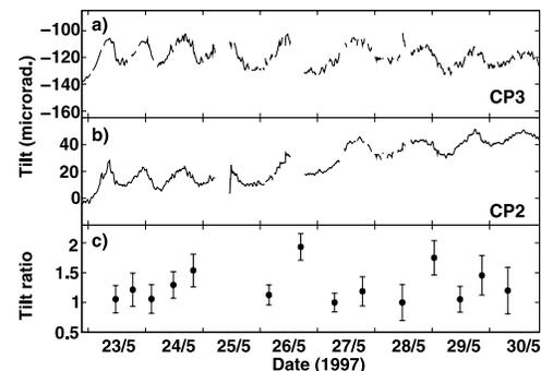
**Figure 3.** Radial tilt records for stations (a) CP3 and (b) CP2 for May 23rd to 30th 1997, the only period that the two stations are recording simultaneously. (c) The tilt ratios,  $\theta_{CP3}/\theta_{CP2}$ . The error bars reflect the uncertainty in maxima/minima measurements due to noise inherent on the records. Data gaps are due to loss of signal transmission from the instruments.
