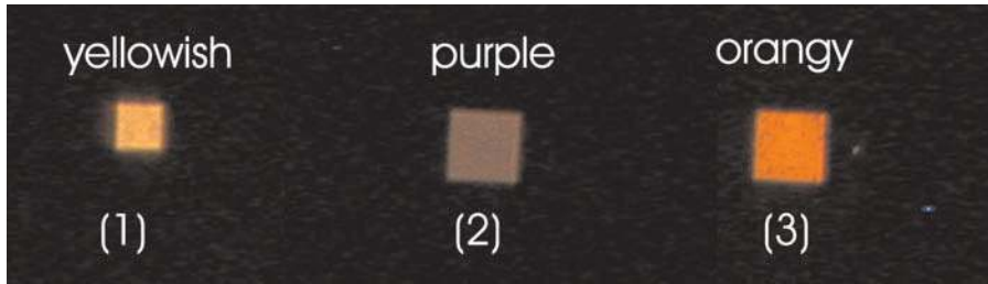
Fig. 2. Far field image of three different AAAs in real colours obtained by conventional microscope working in transmission mode. The AAAs are engraved on a 100-nm thick silver layer. The inner diameter ( d_i ), the outer diameter ( d_o ) and the period p are d_i = 100 nm, d_o = 200 nm, p = 350 nm for matrix (1) ( 7 \times 7 \mu\text{m}^2 ); d_i = 230 nm, d_o = 330 nm, p = 500 nm for matrix (2) ( 10 \times 10 \mu\text{m}^2 ) and d_i = 100 nm, d_o = 200 nm, p = 500 nm for matrix (3) ( 10 \times 10 \mu\text{m}^2 ).
