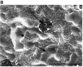
Fig. 6. Fracture surfaces of specimens oxidized 100 1 h-cycles at 1100 °C prior to adhesion test. (A) AM1/ $\beta$ -NiAl(Zr)/YPSZ. (B) AM1/ $\beta$ -(Ni,Pt)Al/YPSZ.
