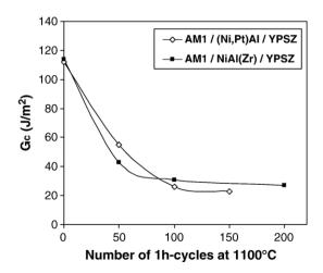
Fig. 5. Adhesion energies  $G_{\rm c}$  of two TBC systems, as a function of the number of 1 h-cycles at 1100 °C. (3 to 5 specimens tested for each result; typical dispersion around 10%).
