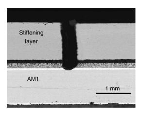
Fig. 2. Partial view of a modified notched four-point bending specimen.
