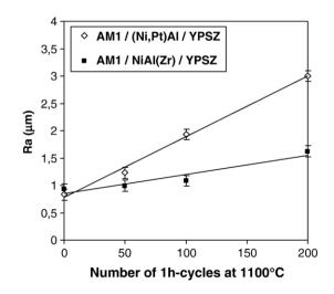
Fig. 7. Arithmetical mean roughness (Ra) of the TGO/bond coat interface of two TBC systems as a function of the number of 1 h-cycles at 1100 °C.
