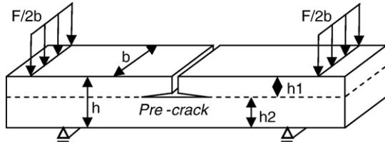
Fig. 1. Four-point bending specimen with symmetrical interfacial cracks [2].
