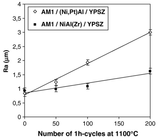
Fig. 7. Arithmetical mean roughness (Ra) of the TGO/bond coat interface of two TBC systems as a function of the number of 1 h-cycles at  $1100 \text{ }^\circ\text{C}$ .
