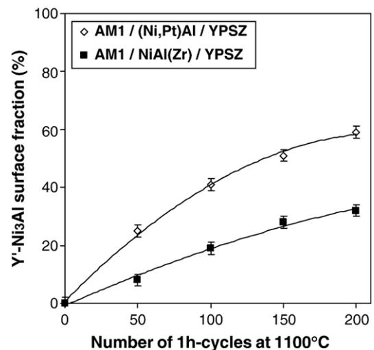
Fig. 9. Evolution of the surface fraction of the  $\gamma'$ -Ni<sub>3</sub>Al phase in the bond coats of two TBC systems as a function of the number of 1 h-cycles at 1100 °C.
