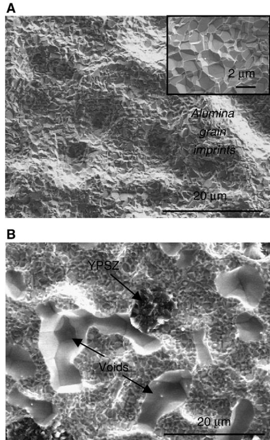
Fig. 6. Fracture surfaces of specimens oxidized 100 1 h-cycles at  $1100 \text{ }^\circ\text{C}$  prior to adhesion test. (A) AM1/ $\beta$ -NiAl(Zr)/YPSZ. (B) AM1/ $\beta$ -(Ni,Pt)Al/YPSZ.
