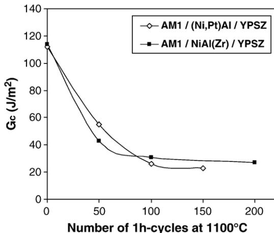
Fig. 5. Adhesion energies  $G_c$  of two TBC systems, as a function of the number of 1 h-cycles at  $1100 \text{ }^\circ\text{C}$ . (3 to 5 specimens tested for each result; typical dispersion around 10%).
