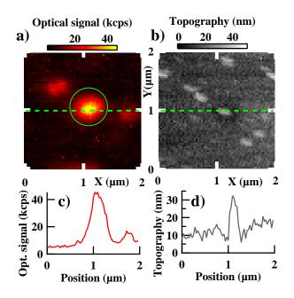
Fig. 1. NSOM detection of a single NV color center in a nanodiamond. (a) Luminescence image recorded with an excitation optical power of 100  $\mu$ W at the tip apex. Integration time: 140 ms per pixel, scan speed: 0.5  $\mu$ m.s<sup>-1</sup>. (b) Corresponding topography. The image has been numerically flattened. (c) (resp. (d)) Line cut along the green dashed line of images (a) (resp. (b)).
