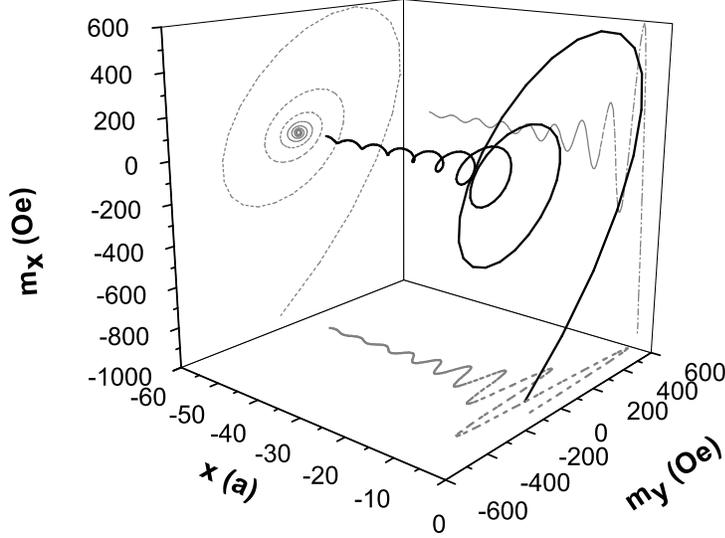
**Figure 14.** Transfer spin density (black line) as a function of the distance in the left ferromagnetic electrode in a strong ferromagnetic regime. We set  $\epsilon^\perp = -0.38$  eV and  $V_b = 0.1$  V.
