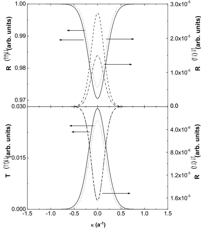
**Figure 3.** Reflectivity (top panel) and transmittivity (bottom panel) as a function of  $\kappa$ . The solid and dotted lines represent the spin conserving reflectivity and transmittivity for initially majority and minority spins respectively (left axes); the dashed and dotted-dashed lines represent the mixing reflectivity and transmittivity for initially majority and minority spins respectively (right axes). The applied bias voltage is  $V_b = 0.1$  V and  $\theta=90^\circ$ .
