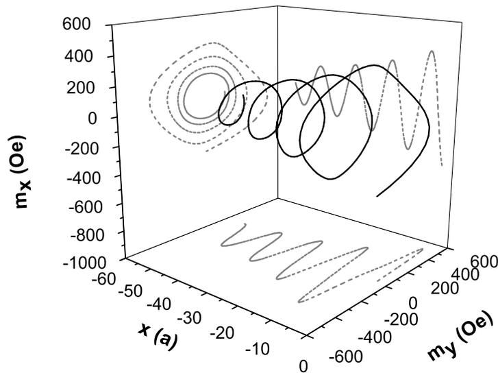
**Figure 13.** Transfer spin density (black line) as a function of the distance in the left ferromagnetic electrode in a usual ferromagnetic regime. We set  $\epsilon^\perp = -1.37$  eV and  $V_b = 0.1$  V.
