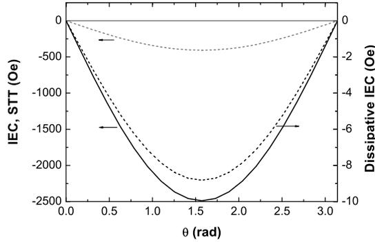
**Figure 7.** Angular dependence of spin transfer (grey) and interlayer exchange coupling (black): conservative part (at zero bias - solid lines) and dissipative parts (bias dependent part - dashed lines). The dissipative parts are calculated at  $V_b = 0.1$  V.
