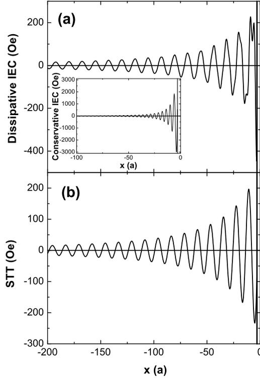
**Figure 8.** Total spin density as a function of the location in the left electrode: a) Current-induced interlayer exchange coupling - inset: Interlayer exchange coupling at zero bias voltage; b) Spin transfer torque. These quantities are calculated at  $V_b = 0.1$  V.
