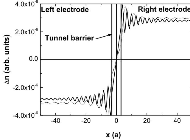
**Figure 9.** Out-of-equilibrium longitudinal spin density along the magnetic tunnel junction for majority (solid line) and minority (dotted line) electron spin projections. The bias voltage is  $V_b = 0.1$  V.
