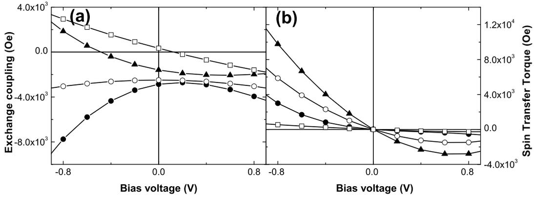
**Figure 11.** Bias dependence of interlayer exchange coupling (a) and spin transfer torque (b) for  $J_{sd} = 1.62$  eV and different values integration depth:  $t = 0$  Å (open squares),  $t = 4$  Å (filled triangles),  $t = 10$  Å (filled circles),  $t = \infty$  Å (open circles).
