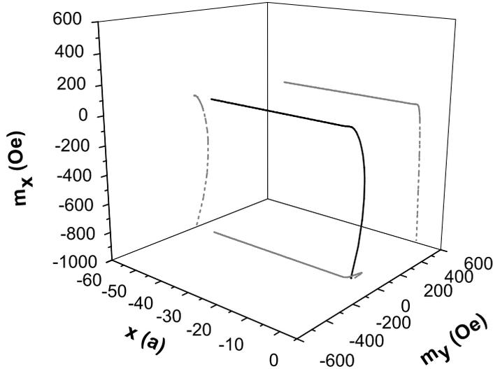
**Figure 15.** Transfer spin density (black line) as a function of the distance in the left ferromagnetic electrode in half-metallic regime. We set  $\epsilon^\perp = 19$  eV and  $V_b = 0.1$  V.
