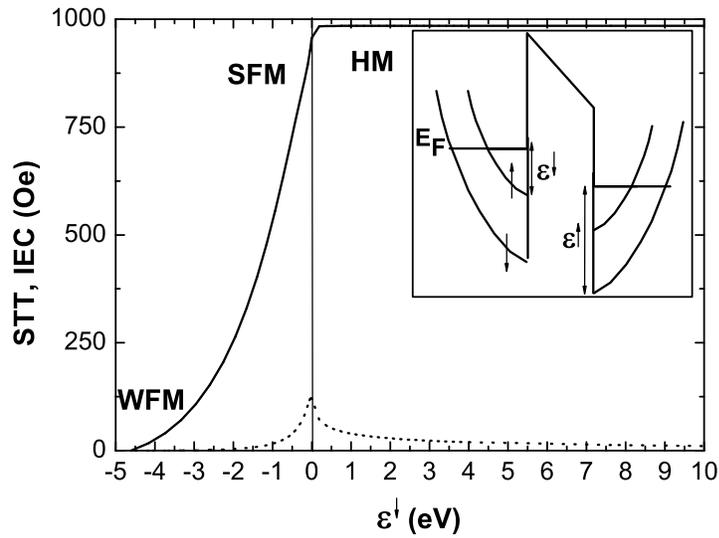
**Figure 12.** Spin transfer torque (solid line) and dissipative interlayer exchange coupling (dotted line) as a function of  $s$ - $d$  exchange coupling. The vertical line shows the limit between ferromagnetic (weak ferromagnetic -WFM- and strong ferromagnetic -SFM-) regime and half-metallic regime.
