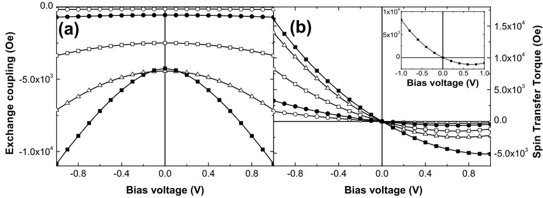
**Figure 10.** Bias dependence of interlayer exchange coupling (a) and spin transfer torque (b) for different values of  $s$ - $d$  coupling:  $J_{sd} = 0.38$  eV (open circles),  $J_{sd} = 0.76$  eV (filled circles),  $J_{sd} = 1.62$  eV (open squares),  $J_{sd} = 2.29$  eV (open triangles),  $J_{sd} = 2.97$  eV (filled squares). Top inset: Bias dependence of STT for  $J_{sd} = 1.62$  eV; the solid line was calculated following the usual way and the symbols were calculated using Eq. 51.
