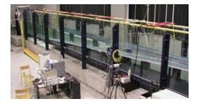
In these experiments a soliton is produced by a wavemaker. It propagates along a mild slope (1/15) up to breaking. Instead of the previous initial free surface, we used the following one  $y = h + Ae^{-R(x-L)^2}$  For L = 2m A = 0.31m, h = 0.122m and R = 4.3, we can reproduce quite accurately the final instant (t = 0.8635s) of the breaking as illustrated below
