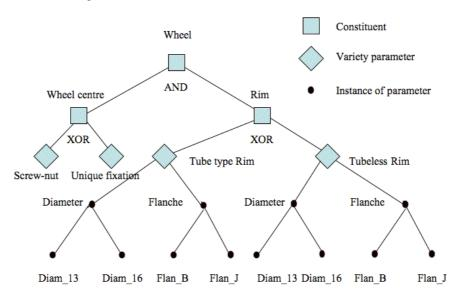
Figure 3: A generic structure representing variety in a wheel family
