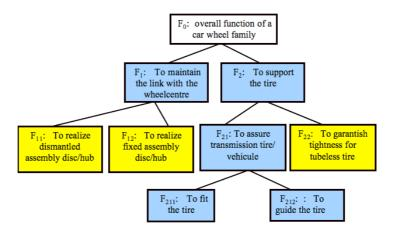
Figure 1: Functional structure of a wheel family
