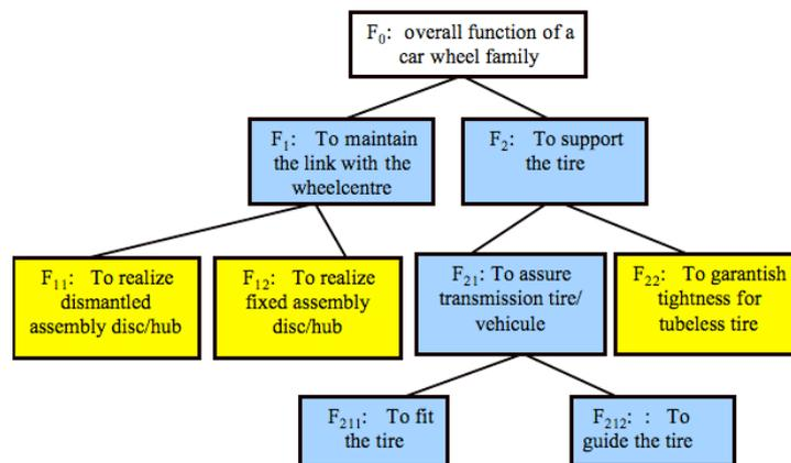
Figure 1: Functional structure of a wheel family
