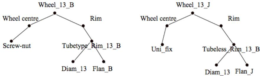
Figure 2: Two examples of distinctive structures of wheels
