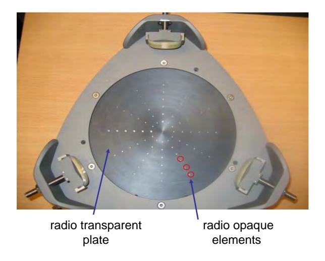
Fig. 3 : The calibration grid is fixed to the image intensifier and contains radio-opaque elements arranged on two parallel plates. Radio-opaque elements who are included in one of the plate (picture) are used to correct the image distortions.
