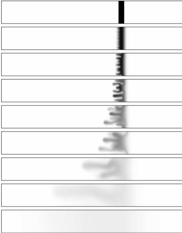
FIG. 2: Density plots of concentration at successive times in the frame moving at the velocity U . From top to bottom: t=0 , 500, 700, 1000, 1500, 2000, 5000, 15000 and 60000 ( Pe = 512 , l = 128 , R = 2 , \varepsilon = 1 ).
