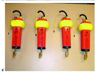
FIG. 1. The three salinity drifters used during the COSMOS experiment: (a) the SIO SVP model (C/T cell on the right side); (b) the METOCEAN SVP model (C/T cell underneath); (c) SURFACT drifters (C/T cell underneath).
