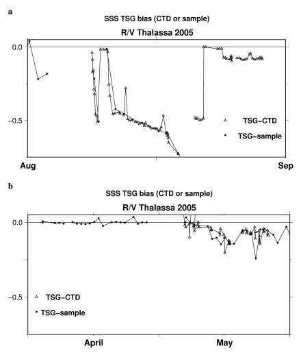
Fig. 2. Comparison of the TSG salinity of the R/V *Thalassa* with CTD 3-m values (triangles) and water samples collected at the TSG (dots) for two periods [(a) mid-August to mid-September; (b) April and May].
