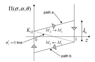
**Figure 6.** Thermodynamical force  $\Pi(\sigma, \alpha, \theta)$  as a function of the  $M_1$  martensite fraction  $z \in [0, 1]$ .
