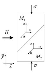
Figure 4. The MSM sample is subject to a compressive stress in the  $\vec{y}$  direction and to a magnetic field in the  $\vec{x}$  direction.
