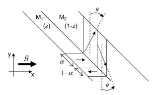
**Figure 1.** Representative Elementary Volume (REV) when the MSM sample is only composed of two martensite variants  $M_1$  and  $M_2$  ( $z = z_1$  and  $1 - z = z_2$ )(Hirsinger and Lexcellent, 2002).
