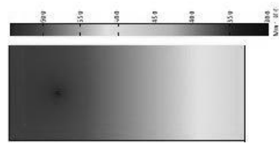
Figure 8 : Finite element modeling of the temperature field around one wire in the 10 μm period case. The top side is on the left.
