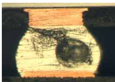
(b) solder joint with void formed away from crack propagation route (void's \phi 140 \mu m fatigue life: 1650cycles)
