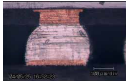
(a) Image of solder joint without void before test
