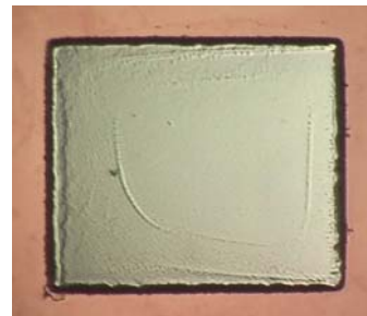
Fig. 10. The gap layer mold. The dimension is 1.15 \times 1.15\text{mm}^2 .
