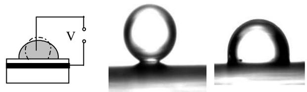
**Figure 1: EWOD principle and pictures of a droplet without and with EWOD actuation.**
