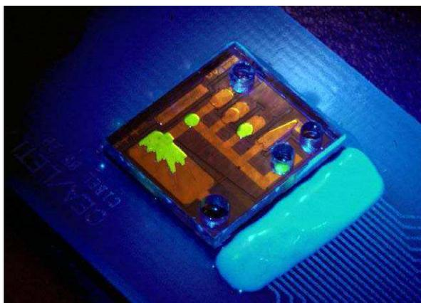
Figure 8: Diagram and photo of closed EWOD chip.
